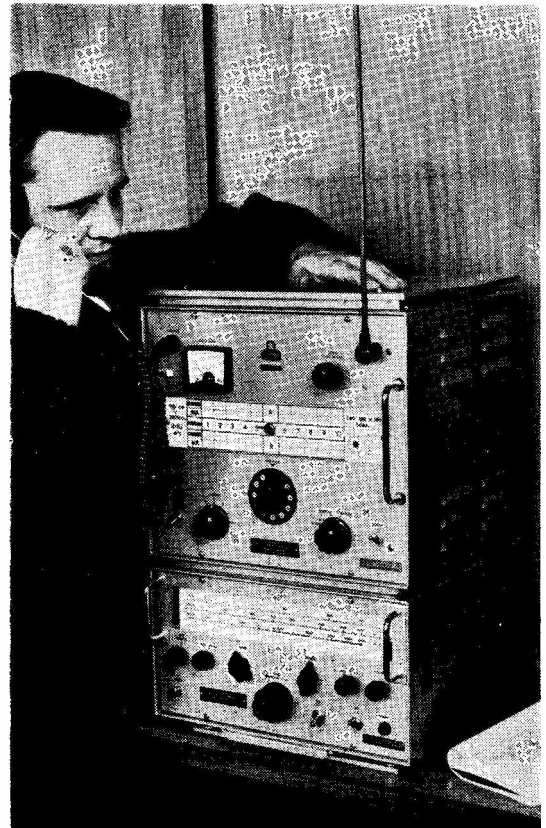
The Marconi Marine Kestrel III Tx/Rx equipment, as used by Sir Francis Chichester to keep in radio contact during his round-world trip "Down the Clipper Way." Courtesy Marconi International Marine Co., Ltd.
